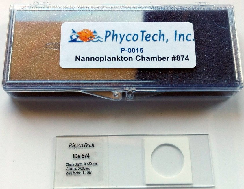
Figure 8. Nannoplankton chamber (86 \mu\text{L} ) used for the observation and monitoring of Gambierdiscus and Fukuyoa cultures.
