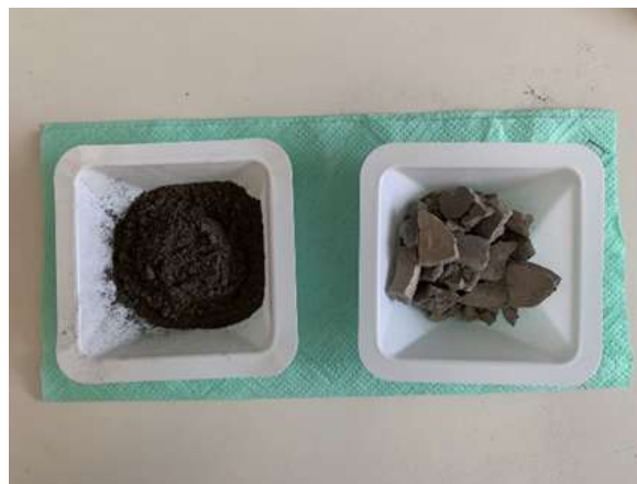
Fig: Produced struvite (left from pig urine and right from cattle urine) containing P_2O_5 , NH_4 and Mg (left) (© A. Beyer, AWI).
