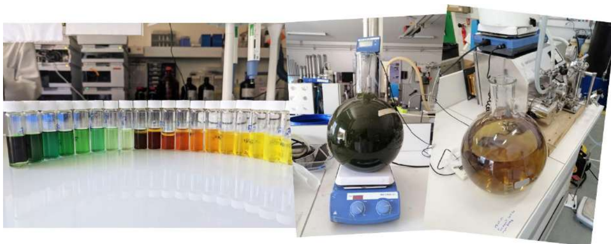
CPC fractions of alcoholic extract on the left, alcalase hydrolysis of the residue in the middle and 10kDa filtration on the right
